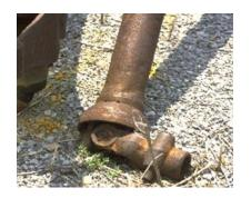
3. Driveline shaft shield is in place but is bent, cracked, sliced, and/or does not rotate freely.
