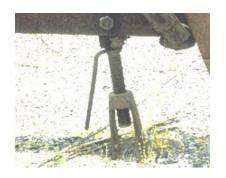
3. Equipment/machine has a jack stand. Jack stand is bent, doesn't sit level on the ground, hand crank is damaged or missing, secured in an up position with a makeshift latch/tie.
