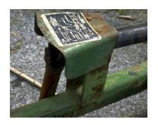
3. Master shield is in place, but has a bend, crack, or slice that reduces the level of protection. Original or current shield offers poor protection.
