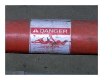
5. Warning decal(s) are mounted on PTO shield or on implement hitch below shaft where they are easily read; includes pictogram.
