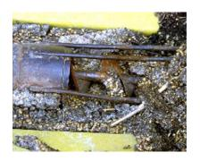
3. Auger has a properly designed intake guard in place but it is bent or damaged; auger has an improperly designed intake guard.
